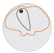
Figure 5. R750 5GHz Elevation Antenna Patterns
