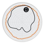
Figure 3. R750 5GHz AzimuthAntenna Patterns
